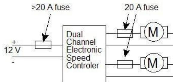
Figure 9: Circuit Protection
