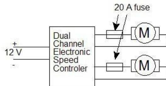
**Recommended Circuit Protection: (ESC IS protected by fuse)**
